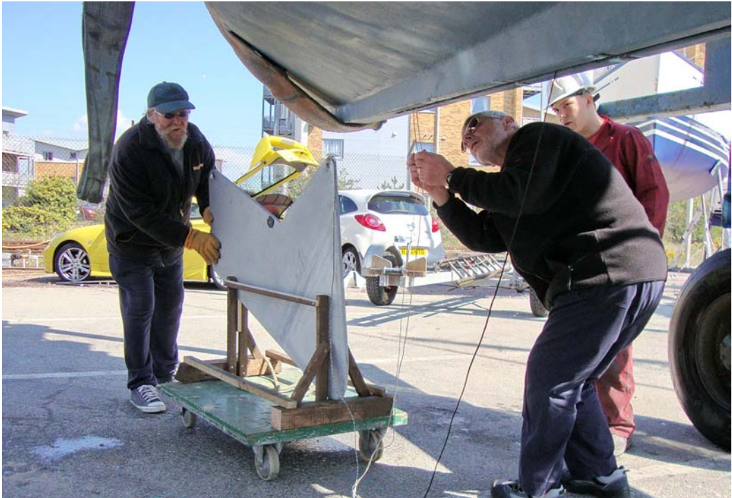
Fig 18: Plate brought to boat & guide lines attached
