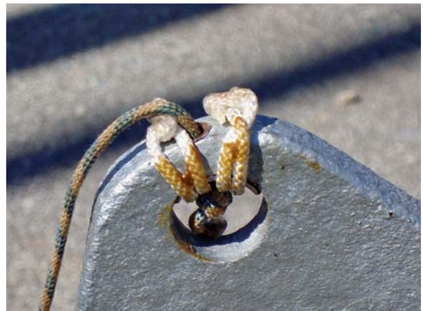
Fig 15: Support saddle in place with Dyneema lifting line & buffer lashings
