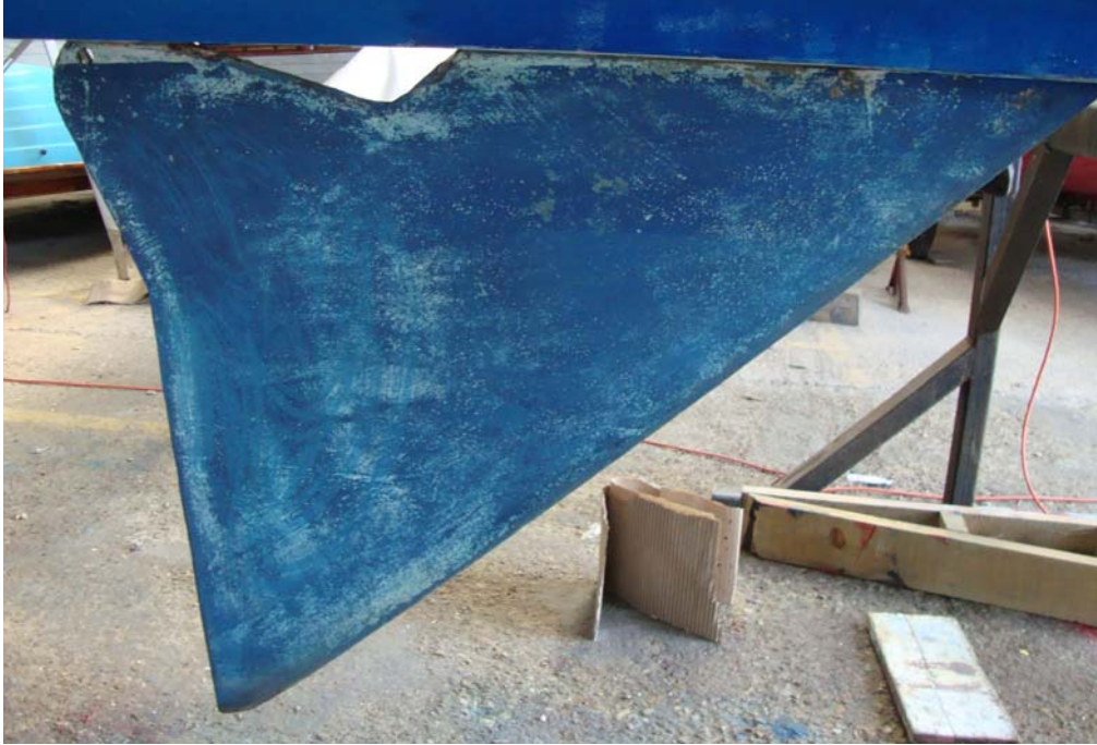
Fig 4: Mk2 centreplate lowered to full extent
