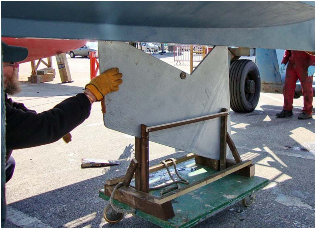
Fig 20: Lower away - fore & aft plate tips enter the slot
