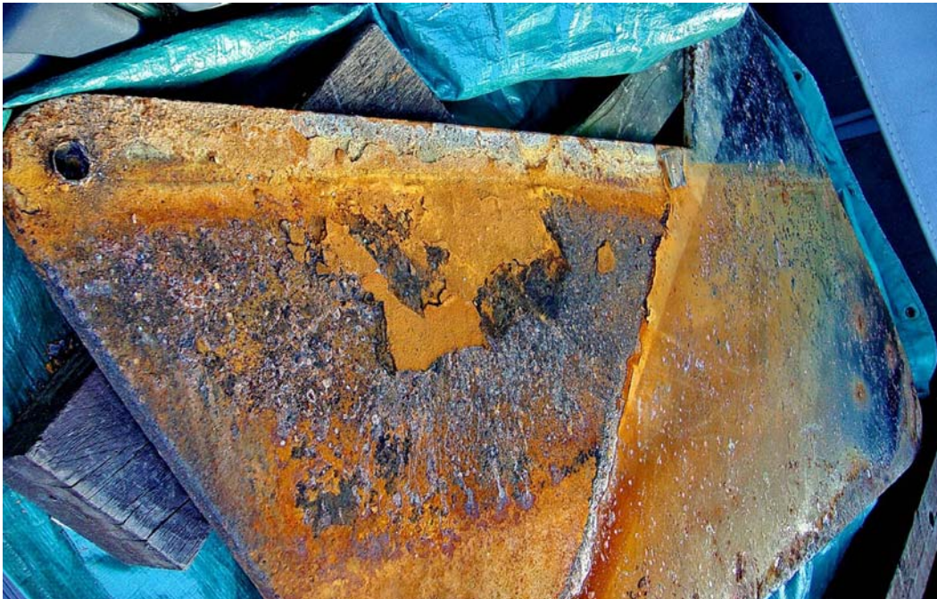
Fig 1: Centreplate as removed
