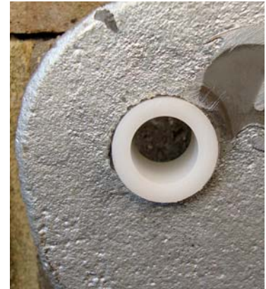
Fig 10: New bush fitted
