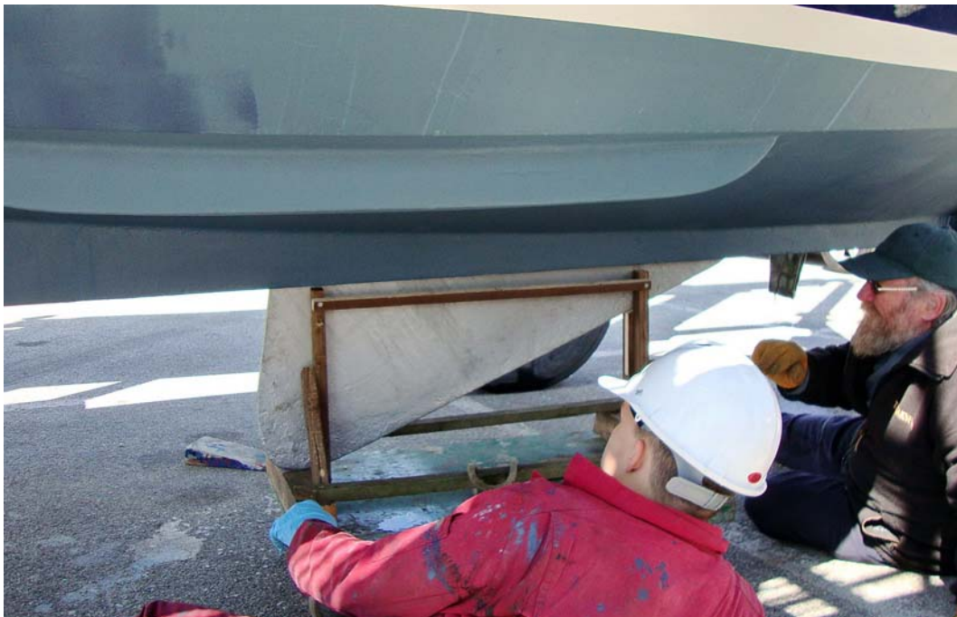
Fig 23: Plate fully in & pivot bolt being fitted. Note small clearance between support frame uprights & underside of keel.
