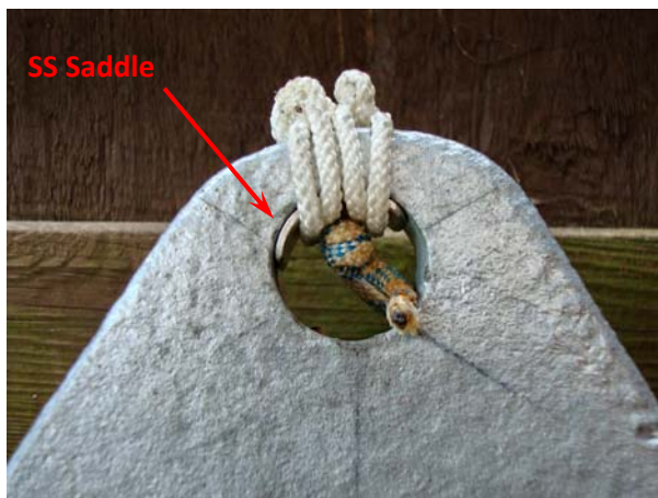
Fig 15: Support saddle in place with Dyneema lifting line & buffer lashings
