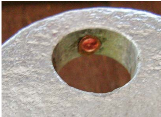
Fig 13: Copper tube hole liner underside
