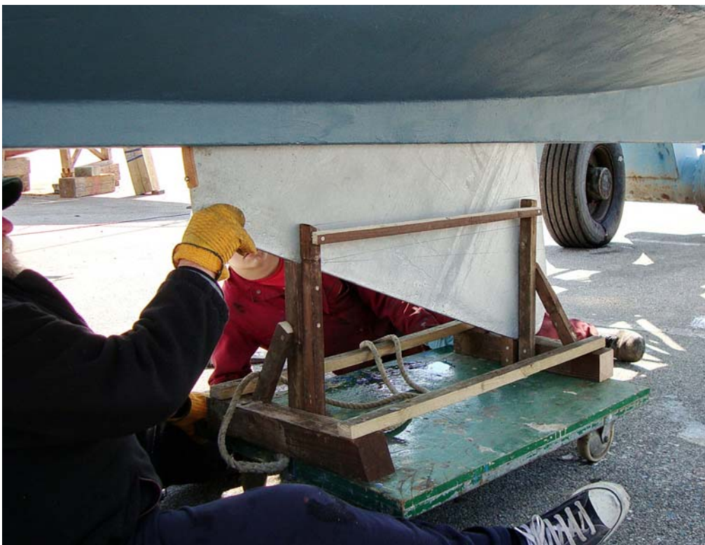
Fig 21: Half way in - forward edge buffer just entering slot
